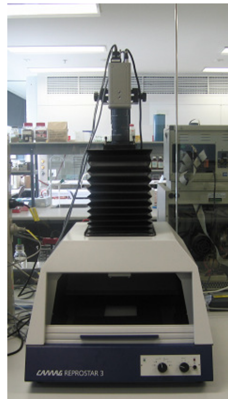
DigiStore 2 documentation system with high- resolution 12-bit CCD camera (HV-C20A, Hitachi, Japan)
